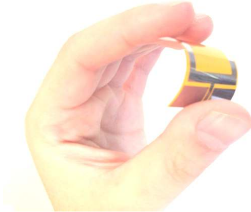
Figure 1. Flexible printed monopole antenna based on Kapton Polyimide substrate.
