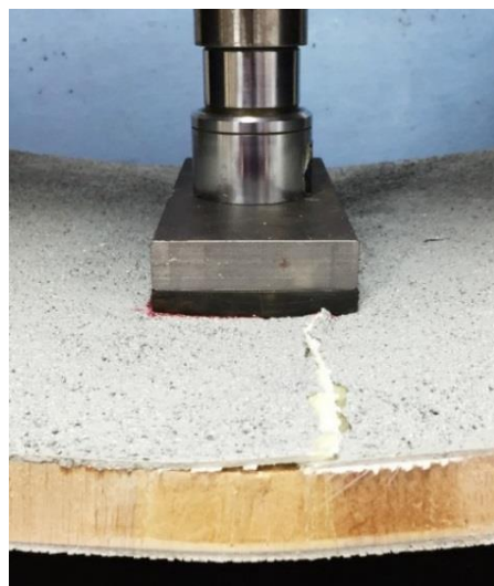
Figure 17. Top face sheet failure observed during large panel testing of 30 mm thick woven GFRP-balsa (SB.150) (single shot) sandwich panel with non-slip coating. Failure propagates along one edge of the rubber pad that simulates a forklift wheel.
