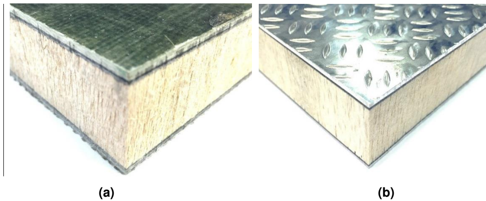
Figure 10. (a) Woven GFRP-balsa (SB.150) sandwich panel (2.1 mm thick face sheets and 25.4 mm thick core). (b) Aluminium-balsa (SB.150) sandwich panel (1.5 mm thick 5052 H32 tread plate top face sheet, 1.2 mm thick 6082 T6 bottom face sheet and 25.4 mm thick SB.150 core). Panels are constructed by bonding the face sheets to the core with methacrylate adhesive.
