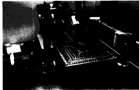
Fig. 17. Laser Doppler Vibrometer (LDV) setup for noncontact interferometric dynamic testing of microgimbals (see [1]).
