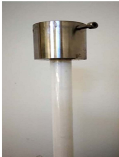
Fig. 5. Sample of 6H-SiC sapphire fiber optic vibration sensor connected with the hollow ceramic tube.
