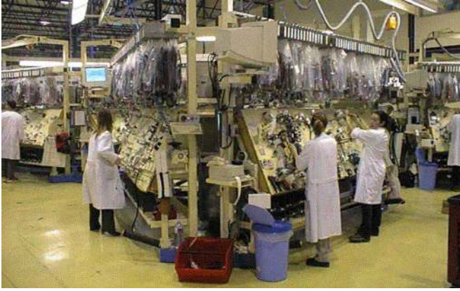
Fig. 2. Final assembly of wire harnesses [7].
