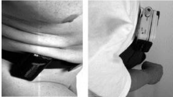
Figure 6, Single point attachment of a common pager or portable stereo is unstable and perceptually separate from the body.
