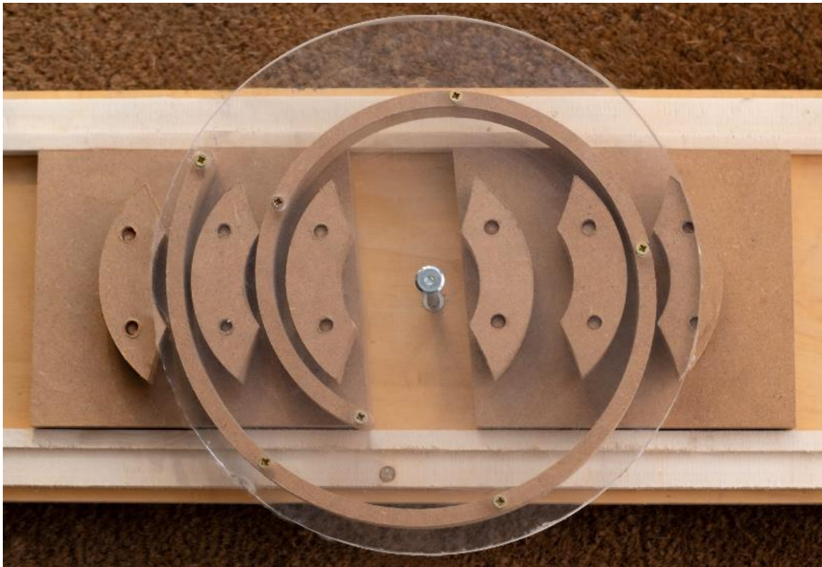
Fig. 15. Larger scale model of a slidable rack driven via rotary cam with a spiral (15 times enlarged)
