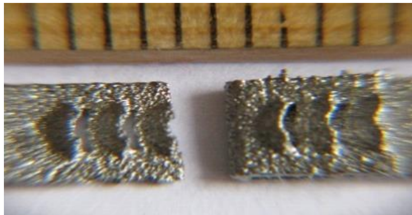
Fig. 13. Fastener's rack made using the 3D SLA printing method from titanium powder (note: the millimetre gradation scale is shown in the top part of the picture)
