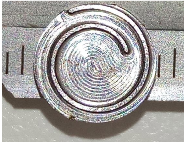
Fig. 14. Rotary cam with a spiral made by machining processes (note: the millimetre gradation scale is shown behind the cam)
