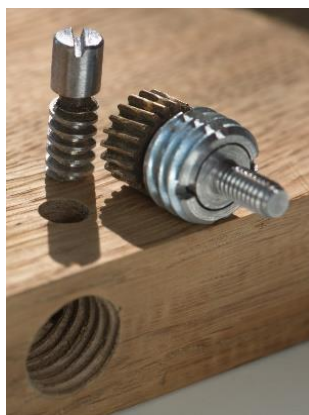
Fig. 6. Innovative fastener S2 based on a worm drive (1 - worm screw, 2 - worm wheel, 3 - axis of worm wheel, 4 - wheel bearing coupler, 5 - fastener coupler, 6 - worm bearing)
