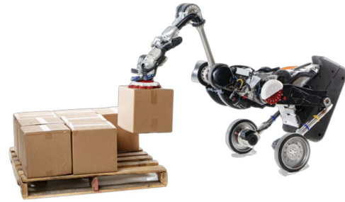
Fig. 2. Mobile mechanoid robot for moving boxes in a warehouse from Boston Dynamics. (Handle robot image provided courtesy of Boston Dynamics, Inc.)
