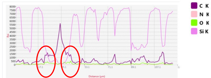
Figure 39: Line based EDX analysis of SiC/Si 3 N 4 /SiC coated sample exposed to 1000 °C for 1 h with increased oxygen content at the edge of fibres bordering a carbon rich zone
