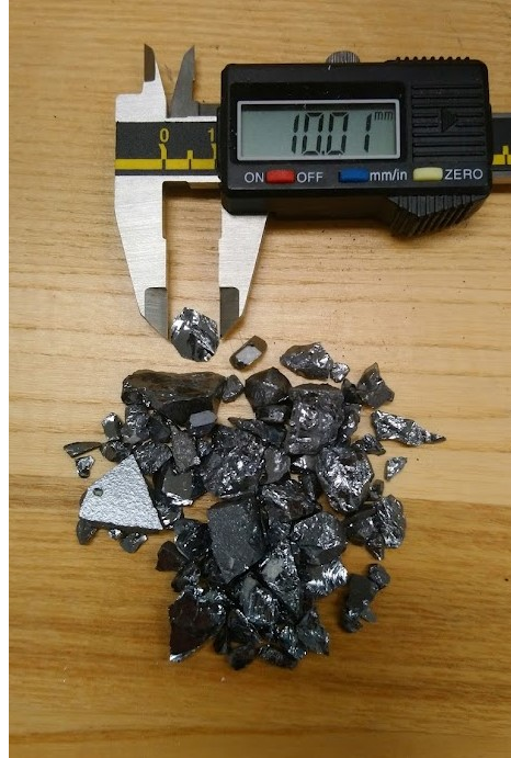
Figure 9: Shaved silicon pellets with micrometer to provide an indication of pellet size
