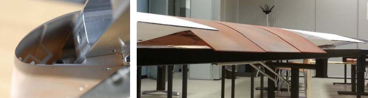
Figure 12 A sketch of the wing model with the assembled morphing LE and TE.
