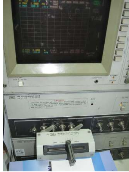
Fig. 9. Experimental setup for electrical characterization of the compact planar transformer.
