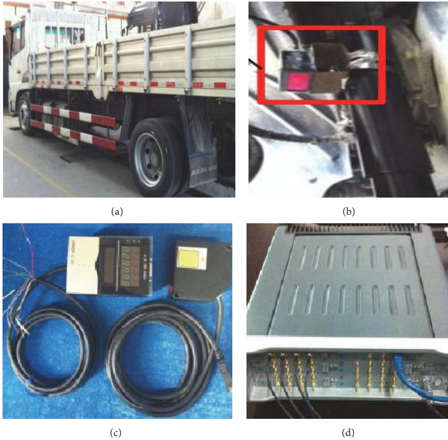
FIGURE 11: The vehicle test for road roughness. (a) The vehicle in the test; (b) the location of sensor on the shock absorber; (c) the displacement sensor; (d) data collection equipment.
