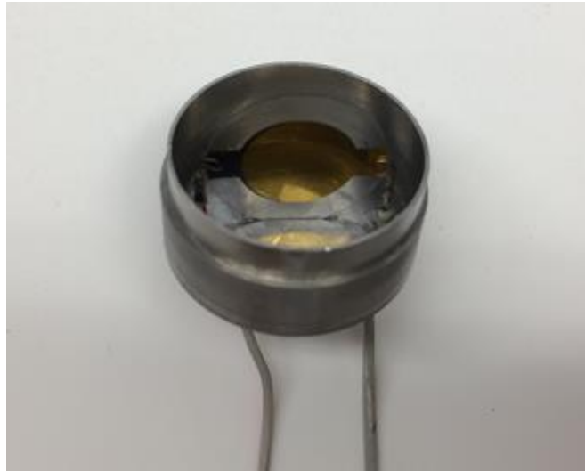
Figure 38: Mounted crystal on one end cap (holder)
