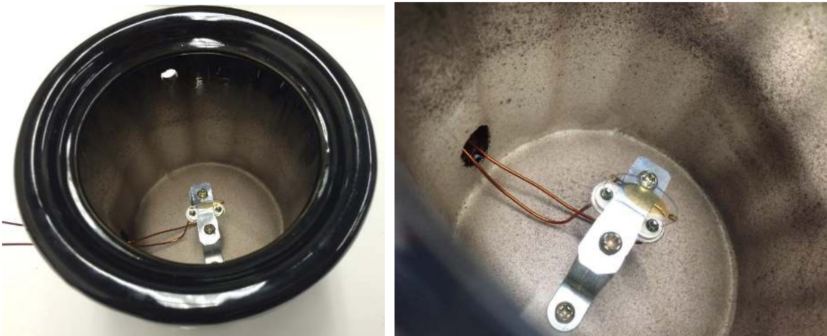
Figure 52: Crystal resonator mounting and connection in the ceramic box
