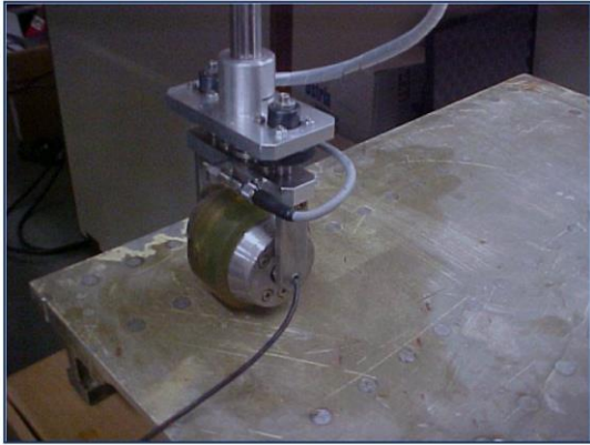
Fig. 10. Wheel probe under test
