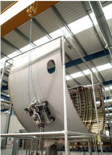
Fig. 11. Robot climbing on a D10 aircraft fuselage section
