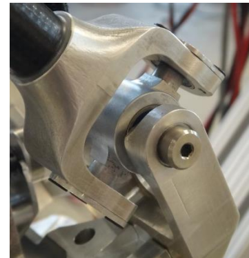
Figure 9: Lower universal joint for the ankle actuators
