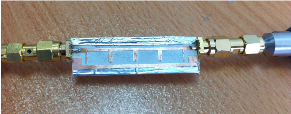
Figure 3.25: The final view of the filter at the final measurement process
