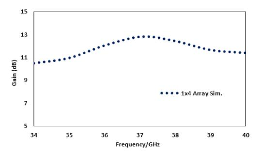
Figure 4. Gain of the four element antenna array.
