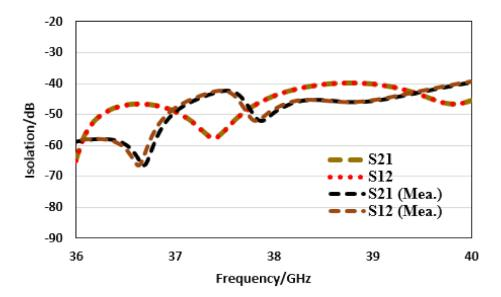
Figure 8. Corporate array MIMO isolation analysis.
