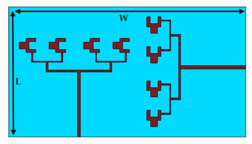
Figure 5. Corporate feed array MIMO configuration.
