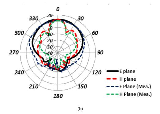
Figure 9. Corporate array MIMO configuration gain pattern for: (a) port-1, (b) port-2.
