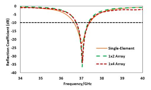
Figure 3. Reflection coefficient comparison for antenna different configurations.
