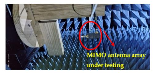
Figure 6. Proposed MIMO antenna array under testing.
