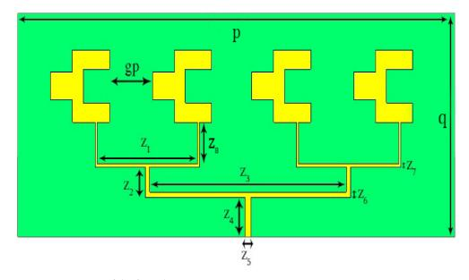
Figure 2. Structure of the four element array antenna.
