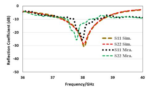
Figure 7. Corporate array MIMO configuration reflection coefficient.
