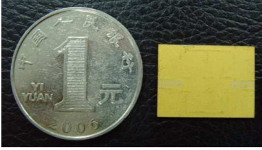
Figure 10. Photo of the fabricated multilayer dual-band double-folded SIW filter.
