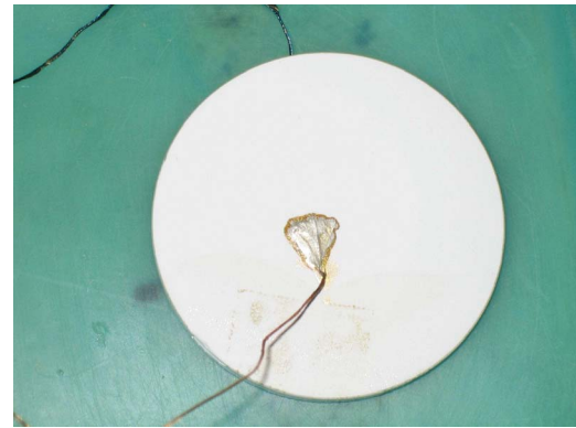
Fig. 11. Disk applied voltage measurement method.
