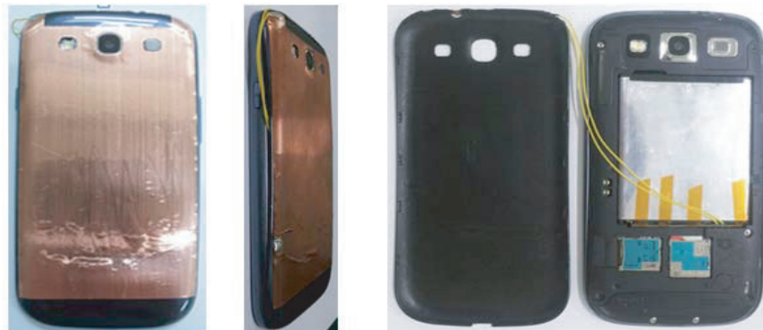
Figure 8. Prototype antenna with a mobile phone.
