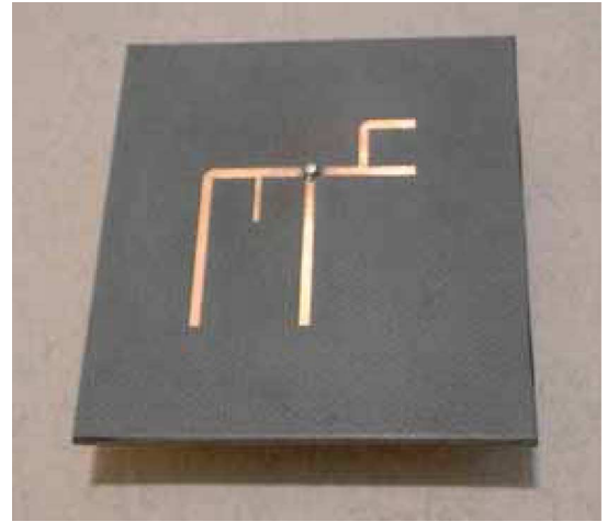
Fig. 6. Boolean PSO-designed antenna element fabricated on RT-Durroid 5880.
