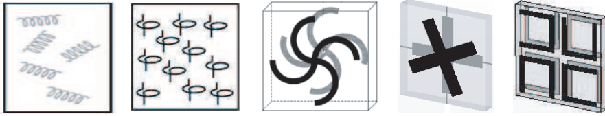
Figure 1. Examples of chiral structures. In analogy to the terminology in chemistry, one can call two chiral (mirror) compounds enantiomorphs, each of them being an enantiomer. Helicity (handedness) is one example of chirality. From left to right, chiral medium based on the random orientation of helical inclusions [17]; uniaxial chiral medium based on oriented wire helices [17]; enantiomeric helicoidal bilayered twisted rosettes [25, 27]; bilayered twisted cut-wire chiral MTM [30, 35, 41]; uniaxial chiral metamaterial constructed by double-layered four “U” split ring resonators [32, 42].
