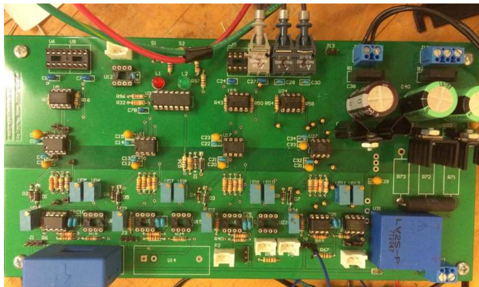
Fig. 6.3. Voltage & Current sensor board.
