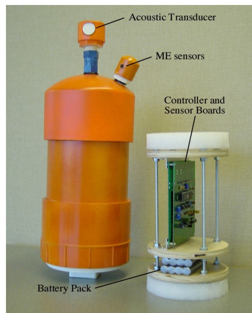
Figure 3a. Photograph of an aqueous sensor network node. The electronics are mounted on a frame (right), which is inserted into the PVC housing of diameter 16.5 cm and length 30.5 cm. The acoustic transducer is mounted at the center top.
