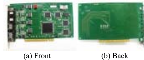
(a) Front (b) Back Figure 13. Quad Force Sensors Interface Board (PCI)
