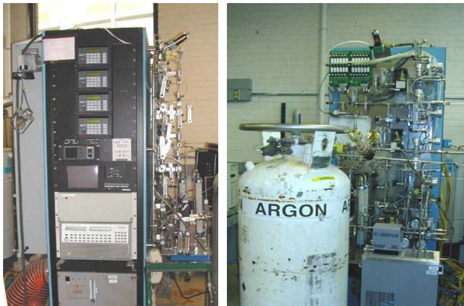
Figure 4.24. (a) A built in gas monitoring /controlling system (b) Side view of (a) with constant temperature water bath.
