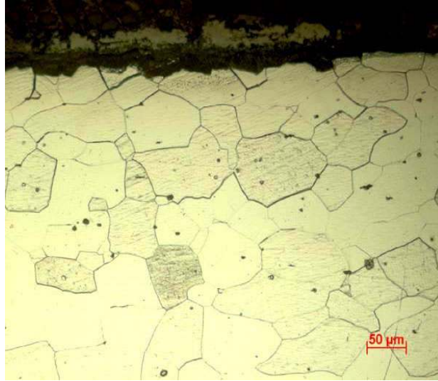
Figure 4.36. Optical micrograph of tested Fe-2.55wt% Si alloy in lead for 100hrs at 600°C - through thickness direction.
