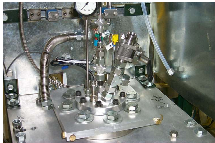
Figure 181. Photograph showing a top view of the corrosion cell containing the oxygen sensors.
