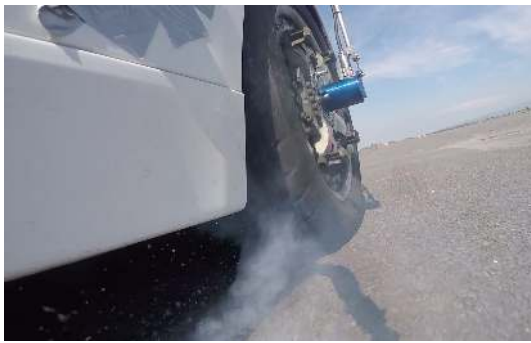
(a) Wheel slip during brake test
