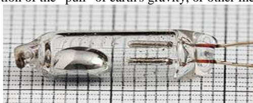
Fig 3: A Single-Pole, Single-Throw (SPST) mercury
