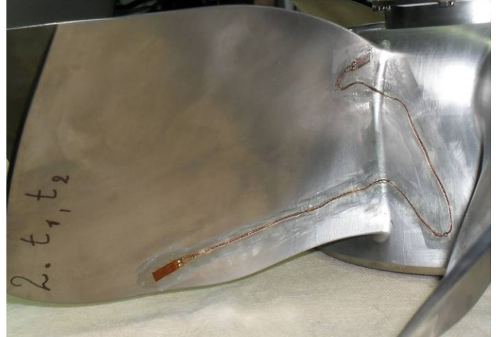
Figure 5: THE INSTRUMENTED STRAIN GAUGES ON THE BLISK1
