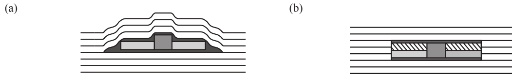
Figure 2. a) Forming embedding technique. b) Cut ply embedding method.
