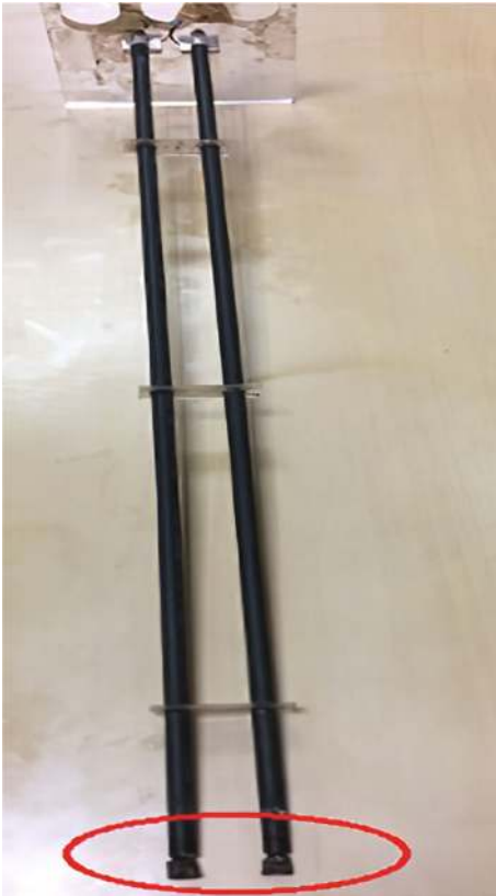
FIGURE 7: Capacitance electrodes for liquid level measurement.
