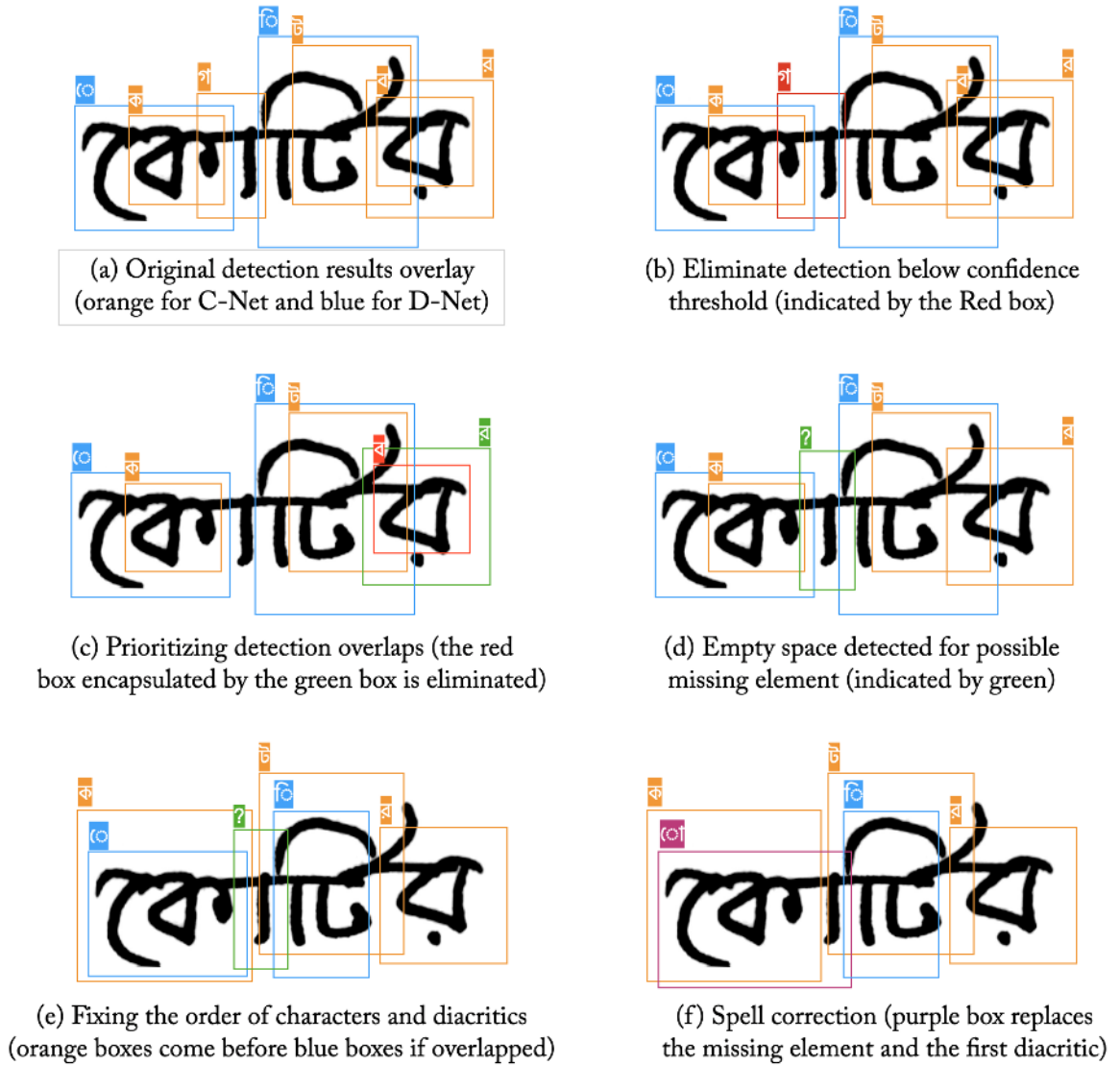
Figure 3.10: Schematic of post processing for Bangla: (a) Original detections, (b) Eliminating detections below threshold, (c) Prioritizing detection overlaps, (d) Allowing empty spaces for possible detection miss, (e) Fixing order of characters and diacritics, (f) Spell correction.
