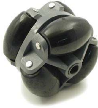
Figure 8.2: the 40 mm radius omniwheel
