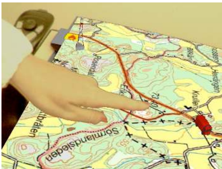
Figure 2: Deictic pointing in a digital map as seen through the head mounted display of the re-designed AR system.
