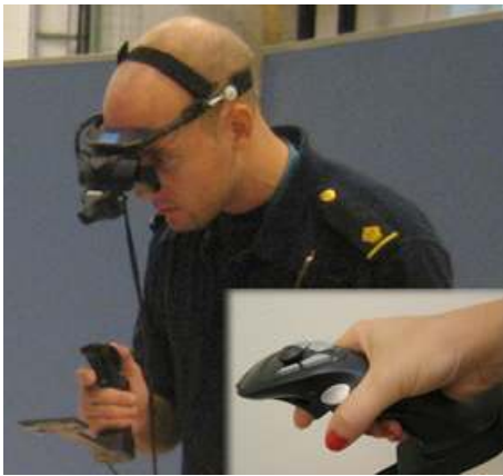
Figure 1: The redesigned display and interaction device, which allows the user to choose a virtual object and place it on the digital map.
