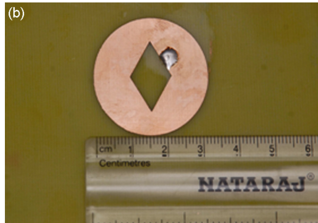
Fig. 3b—View of designed circular patch geometry with concentric diamond slot
