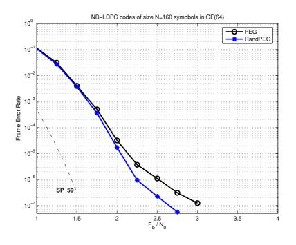
Fig. 1. Performance comparison for the design of non-binary LDPC codes: two codes whose underlying Tanner graphs were constructed with respectively the PEG and RandPEG algorithm are simulated over a BIAWGNC.
