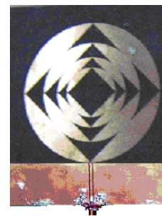
Fig. 8. Photograph of Fourth Iterative Monopole Fractal Antenna
