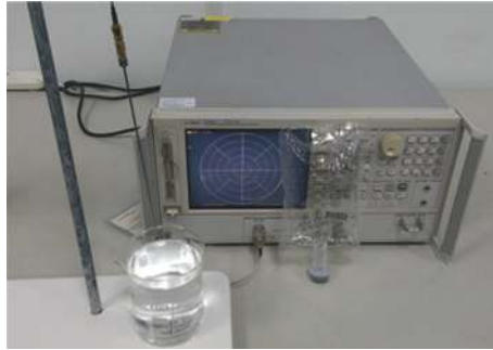
FIGURE 2: IV fluid permittivity and conductivity measurement environment.
