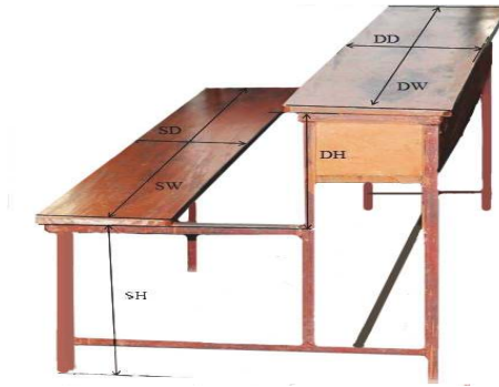
FIGURE 2: Representation of classroom furniture measurements. SD = seat depth, SW = seat width, SH = seat height, DH = desktop height, DW = desktop width, and DD = desktop depth.
