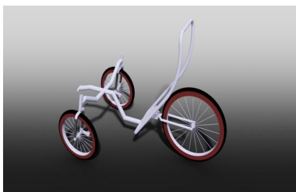
Fig 4.1 HPVC India vehicle without fairing
