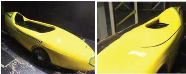
Fig 1.6 Faired vehicles with and without canopy [4]
