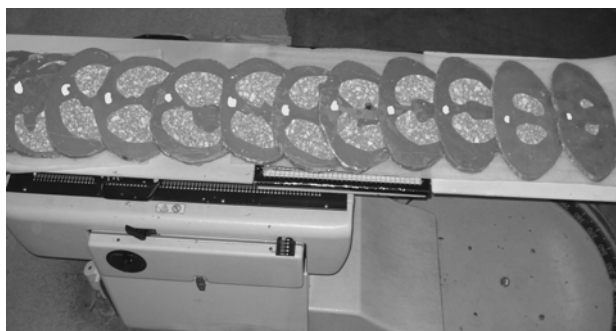
Figure 1. Photograph of slices of heterogeneous thorax phantom, which was created for this study and used for dose measurement and calculation.
