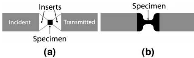
Fig. 3 Additional specimen geometries considered in testing low-ductility materials. (a) Conical inserts, (b) dogbone compression specimen
