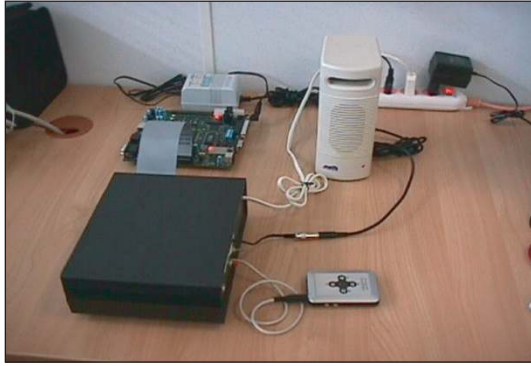
FIGURE 15: System setup for real-time testing of the blind source separation in real time.
