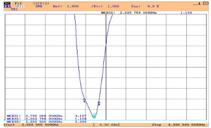
Fig. 14. VSWR of the filter without casing.
