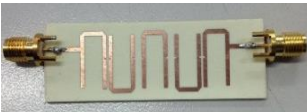
Fig. 7 Actual result of BPF hairpin printed with substrate roger 4350B.
