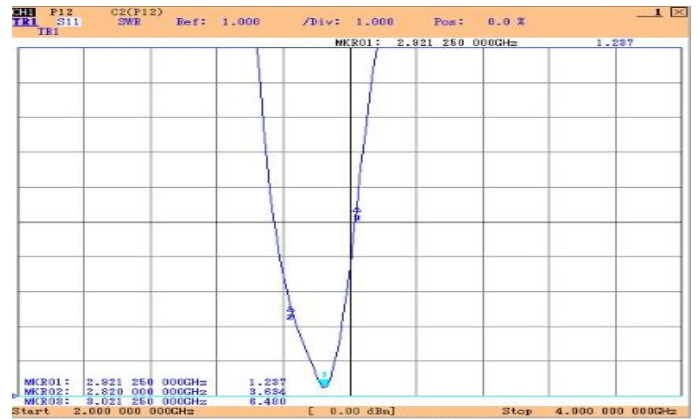
Fig. 15. VSWR of the filter with a casing.
