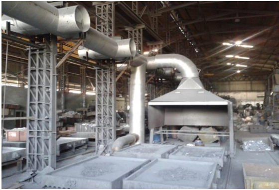
Fig. 2: Actual Photograph of the fume hood
