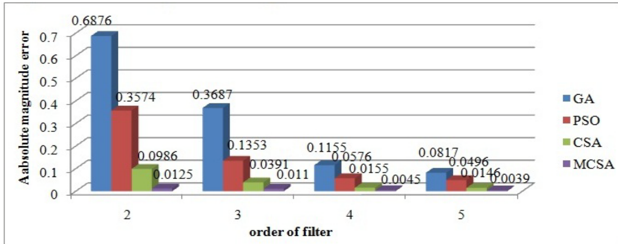
Fig 6: Absolute magnitude error of GA, PSO, CSA and MCSA for filter order 2 nd , 3 rd , 4 th and 5 th .
