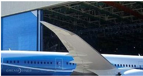
Figure 5 Raked wing tip[14]
