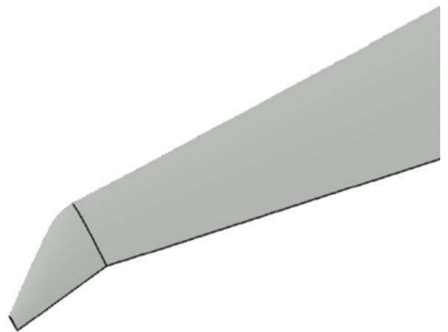
Figure 39 Comparison Boeing 777 winglet with parametric raked winglet
