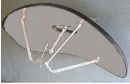
FIGURE 7: Photograph of ring-focus elliptical beam antenna.
