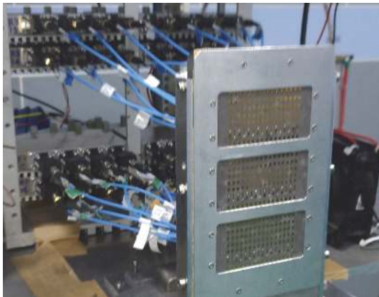
FIGURE 9: The connection of antennas and TR modules.
